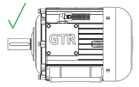
Other installation positions such as vertical installation must not be implemented with our standard generators.
